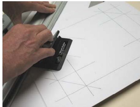
Figure 12: Cut until you reach the stop line and then retract the blade.
