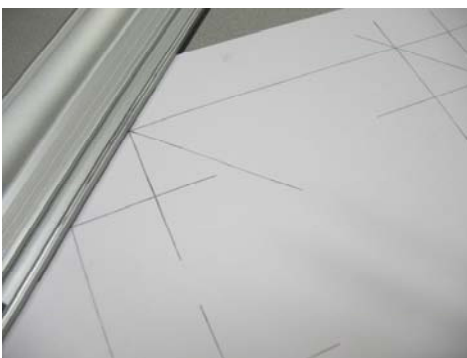
Figure 8: The line you draw will be at a right angle to the 45° angle that bisects the box. This is the key to the whole technique.
