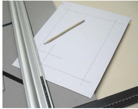
Fig. 3 Align the guide rail of your mat cutter through the box at a 45° angle from corner to corner . Mark a line along the guide rail.
