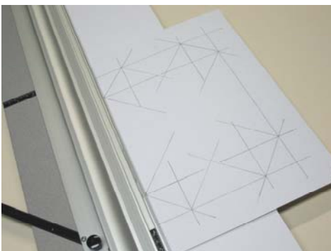
Figure 14: Set the mat guide back to 1/4" and prepare to cut the straight side of the mat's window.
