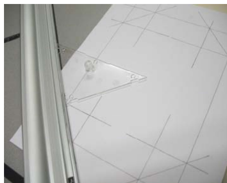
Figure 6: Using a 45/90° triangle, place it so one of the 90° edges is against the guide rail. Position it so the corner of the triangle is at the corner of the penciled square.
