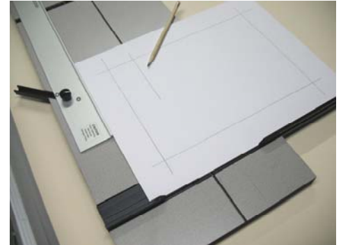
Figure 1: After marking out the borders, measure out along one of the lines 1¾” and draw a line to intersect the first line.
