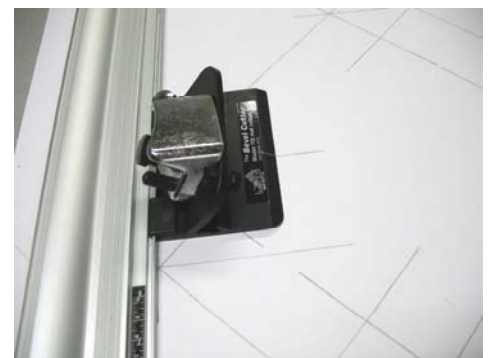
Figure 10: Leave the mat under the guide rail and position the cutting head on the start line.
