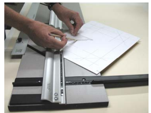
Figure 7: Make a mark along the full length of the 90° side of the triangle.
