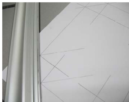
Figure 9: Position the triangle at the opposite corner of the penciled square and extend a line at a right angle from it.
